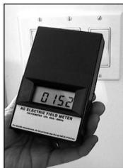
4½-digit readout is in V/m. No conversions necessary.
