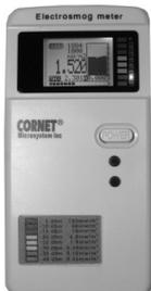
For low cost and versatility, you can't beat this device. It measures both types of low frequency EMF (electric and magnetic fields) plus high frequency radio-waves (micro-waves). Covers a
