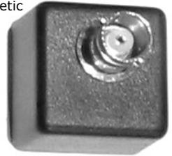
Connect to a display instrument (not included) such as AC voltmeter, oscilloscope or spectrum analyzer to display the output AC voltage and waveform information. These sensors have no minimum measurable field strength, so the sensitivity will depend on your display instrument. Maximum field: the sensor can be damaged above approximately 50 Volts output. Sensor includes operating instructions.
