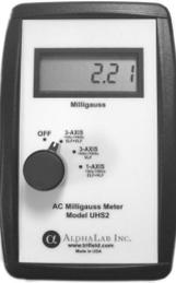
Compact and easy to use, this digital unit can measure ELF and/or VLF magnetic fields in either single axis mode (to help identify the orientation of the field) or 3-axis mode (which makes routine measurements much faster and more reliable).
