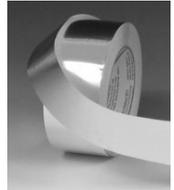
2 mil thick aluminum alloy foil with a pressure sensitive synthetic rubber adhesive and paper liner. The aggressive rubber adhesive sticks well to most surfaces & the paper liner makes for convenient and reliable use.
