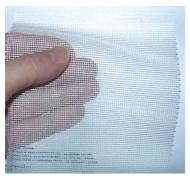
Excellent skin compatible fabric for radiofrequency shielding (cellphones and cell tower radiation, cordless phones, wi-fi, radar, microwave oven leakage, TV broadcast etc). Extremely thin silver coated copper wires are spun with cotton yarn, then woven into washable, comfortable, and durable fabric with the look and feel of normal fabric.
