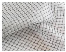
A light weight, durable conductive fabric. Gray BASF Resistat (carbon) fibers woven right into the polyester fabric in an attractive diamond pattern providing surface resistivity of 10<sup>5</sup> ohms per square so it's perfect for static discharge. Very comfortable,
