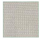
average hole size of less than 1 millimeter provides a whopping 40 dB (99.99%) or better reduction of RF signals from 1 MHz to 2.5 GHz and beyond. Excellent low frequency electric field shielding also. Surface
